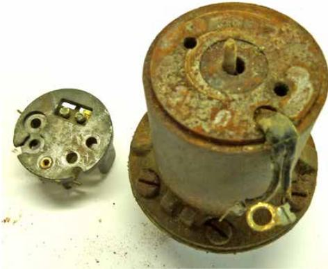
5. With the pedestal removed, turn upside down and remove the steel shaft holding the points to the pedestal.
