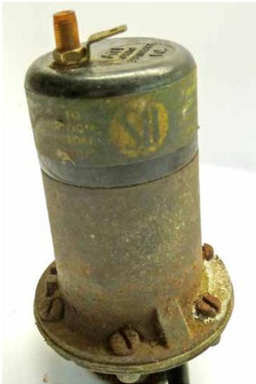
1. Having removed the pump from the car, remove the cap, this requires a small adjustable spanner, not sure what size the nut is, but it isn't a standard UNF size. The nut is holding down the spade connector, star washer and cap.
