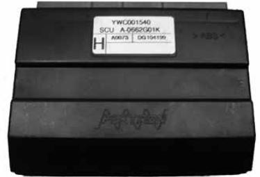
More problematic for the MG owner on a budget (or in the days when these units are no longer available), it appears to be impossible to re-programme a used Pektron SCU if you do not have a matched and working key fob or failing that, the EKA to go with it. The issue here is that the SCU locks out Testbook when the immobiliser is active. Therefore, when a unit fails, it becomes nearly mandatory to purchase a new one unless a used matched fob/EKA and SCU can be found...
