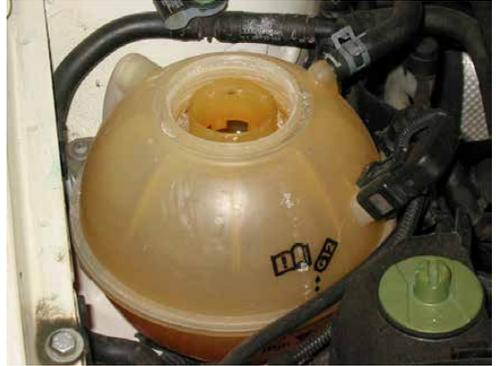
VW Polo double skinned coolant expansion tank
