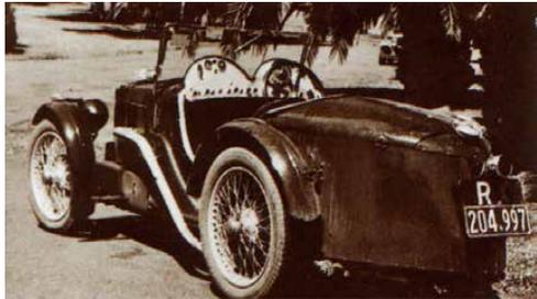
A specially developed twin plate clutch transferred power to the hefty ENV four-speed crash gearbox and the final drive was through straight cut bevel gears. The chassis frame was straight and parallel steel channel which under slung the rear axle and swept over the front axle. Cross-braced tubes passed through the side members and, fixed with brazed flanges, gave a strong yet flexible structure.
