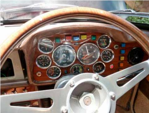
Dash is in but the vacuum gauge isn't working and the rev-counter is over reading, so she has to come out again.
