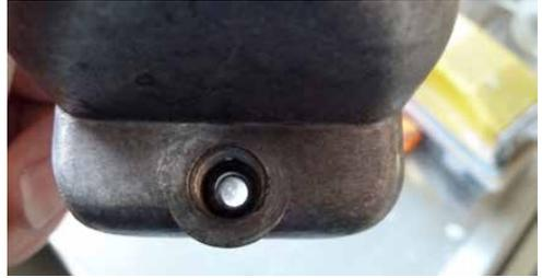
On the home front, 'success' I found the reason for the loss of power. I finally stripped the carburettors and where the LH jet feed goes into the bowl, the hole was restricted from 4mm to 1mm, giving enough fuel for idle and upto 50kph but no more. Once this was cleared the car has been preperforming fine and she is now warranted and registered.
