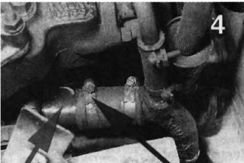
**Step 8.** Disconnect hose connection at the water pump (Photo 4).
