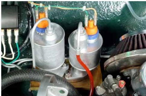
over, fingers crossed no leaks so far. The leak came from a pinhole where the cylinder body meets the reservoir. Impossible to detect until the system is filled and used.
