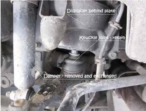
Wheel removed and suspension exposed
