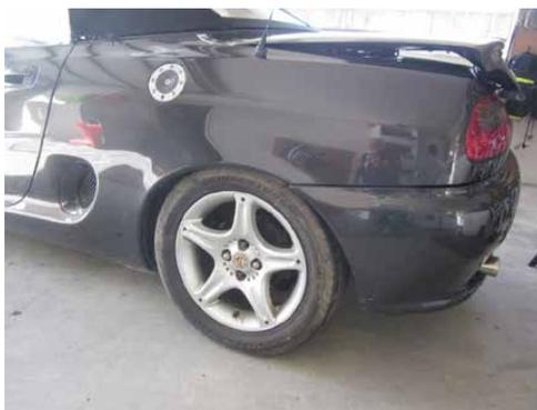
The collapsed suspension
