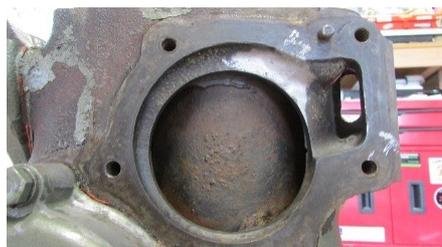
Have just ground away the step on the block casting, where the water-pump is fitted, to improve the water flow and improved the entry channel into the side water gallery. These modifications have been recommended in previous MGC articles and endorsed by the well-respected and much-loved UK MGC Register technical advisor Vic Young and Bruce Ibbotson. Will let you know how we get on. Photo taken after grinding away the webbing in the hole on the right.
